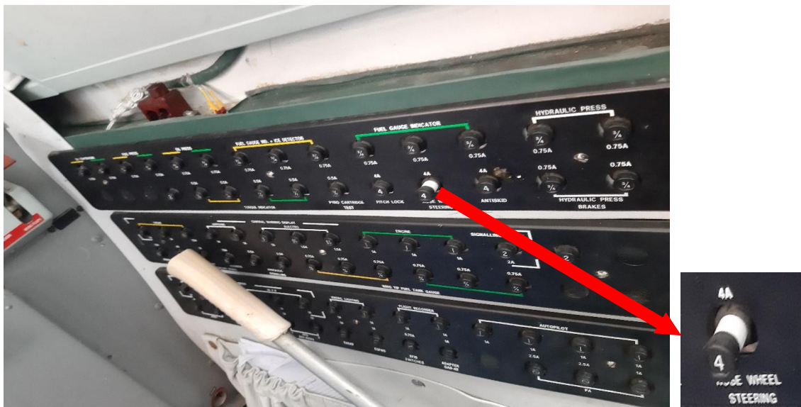
Figure 12 Nose wheel Steering CB was found Popped Out
