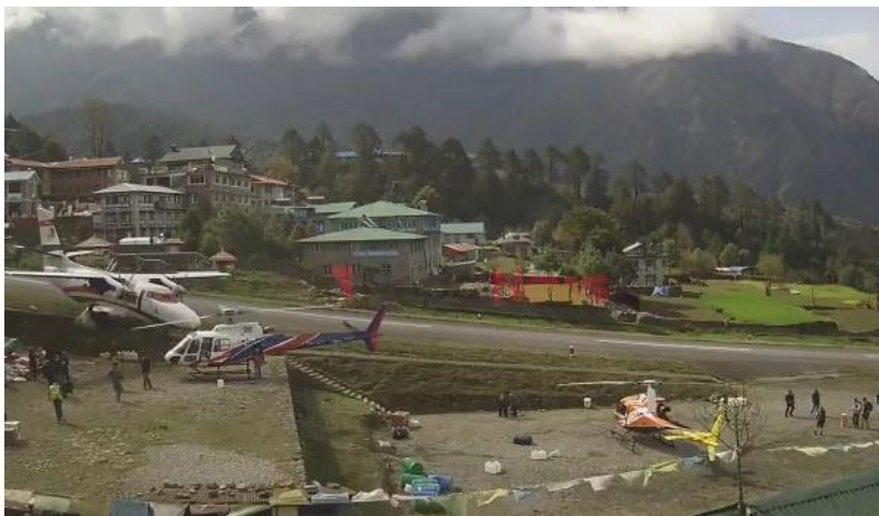
Scene 2 (9N-AMH veered to the right of RWY 24 after 4 secs T/O Roll is initiated)
