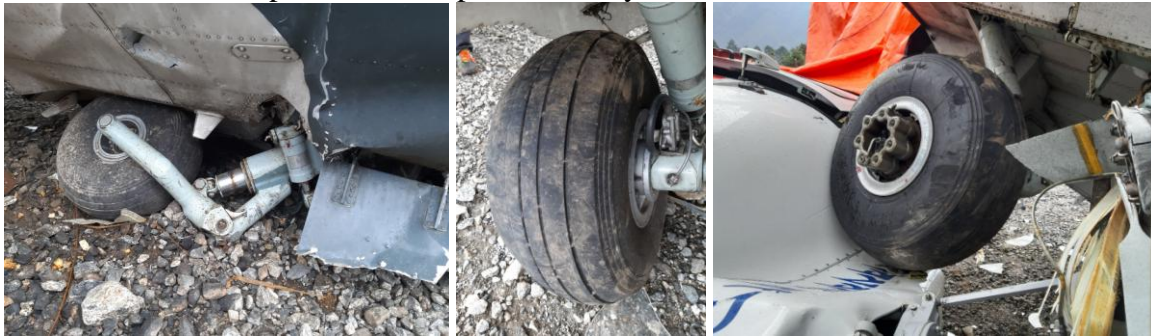
Figure 10 Condition of Nose wheel, LH wheel and RH wheel assemblies
