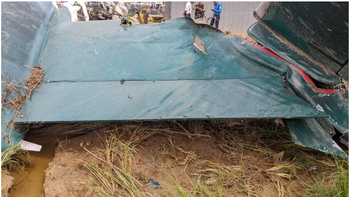
Figure A.7.5: Elevator and rudder deflections as seen at the crash site; top: Elevator in deflected up position, and bottom: rudder in deflected left position
