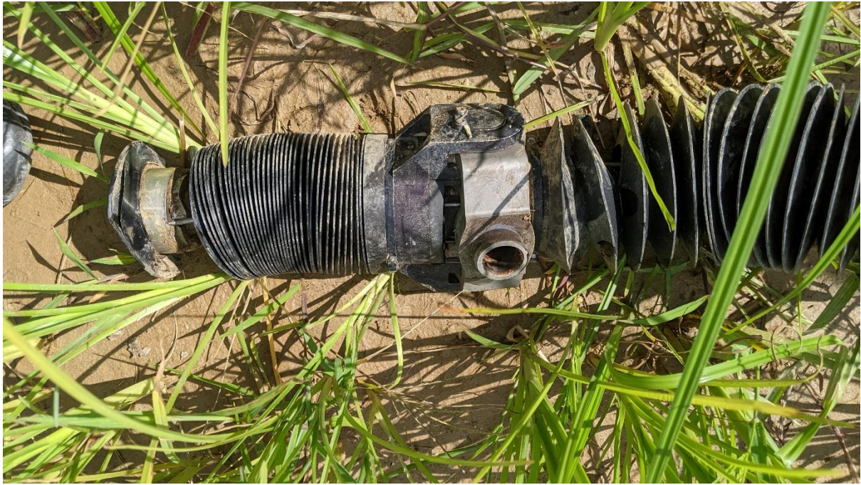
Figure A.7.2: Horizontal stabilizer trim screw
