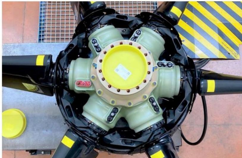
*Figure 21 OEM propeller on Ratier-Figeac assembly line displayed in Feather position*
