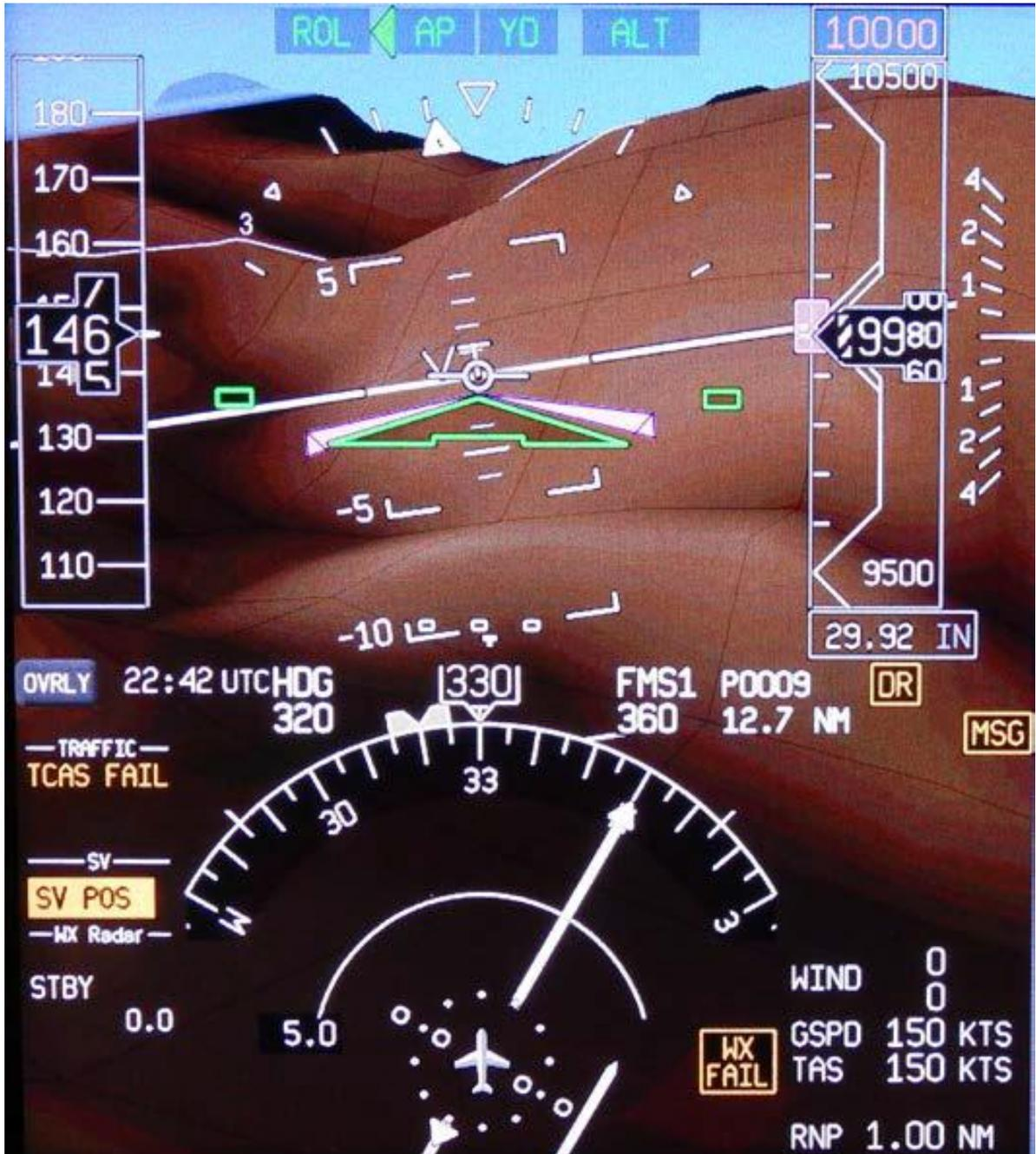
Figure 5. Pilot's Side Display With SVS Enabled at Waypoint P0004
