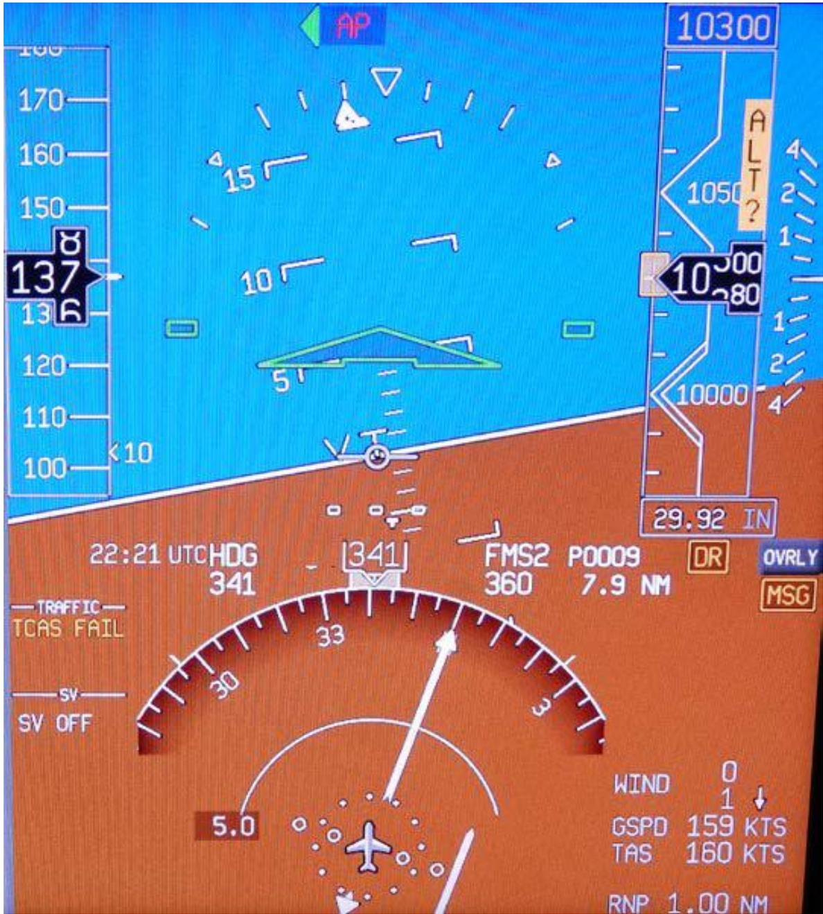
Figure 8. F/O's Side Display Without SVS Enabled at Waypoint P0006
