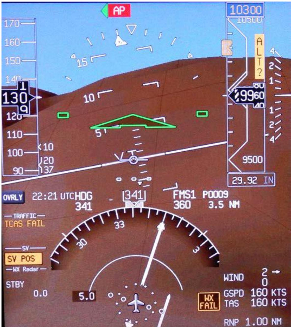
Figure 7. Pilot's Side Display With SVS Enabled at Waypoint P0006
