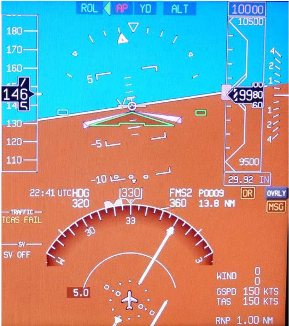
Figure 6. F/O's Side Display Without SVS Enabled at Waypoint P0004
