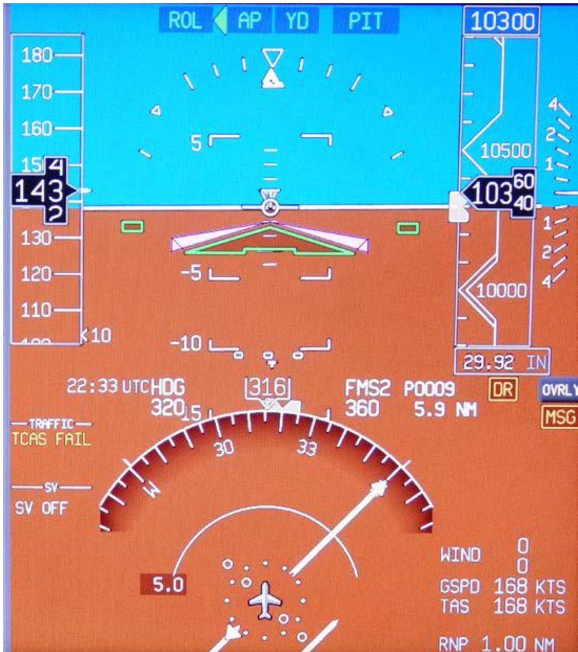
Figure 4. F/O's Side Display Without SVS Enabled at Waypoint P0012
