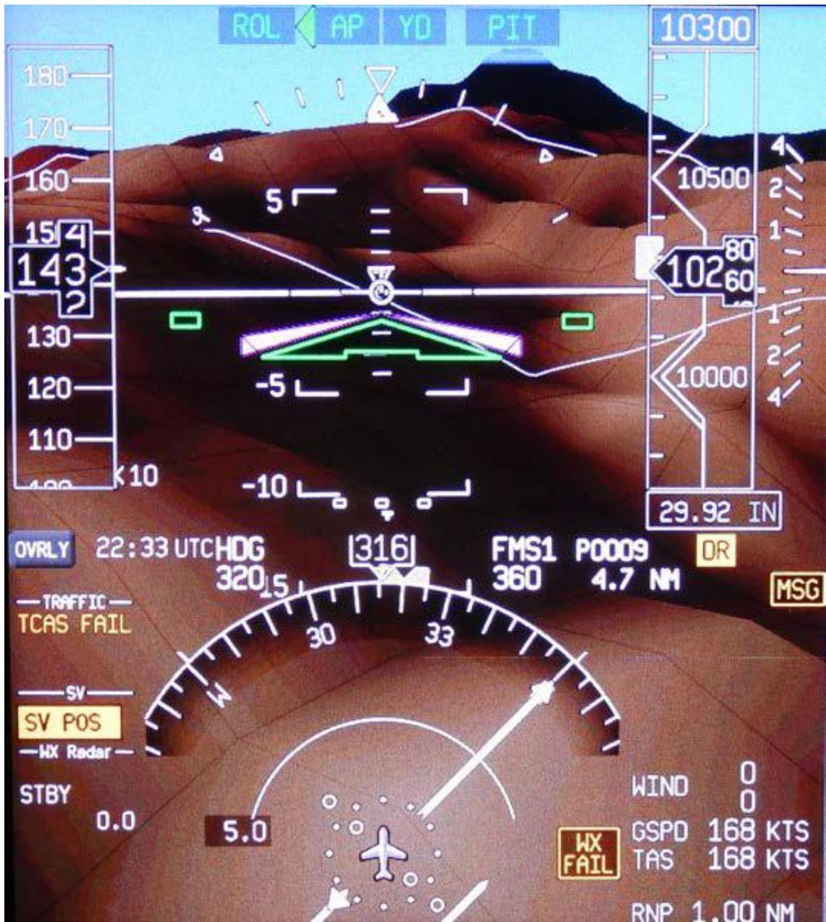
Figure 3. Pilot's Side Display With SVS Enabled at Waypoint P0012
