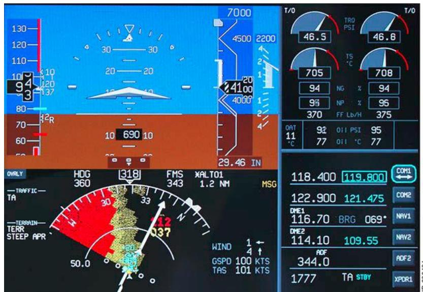
Figure 7: Primary Flight Display (PFD)
