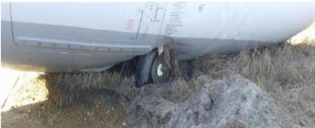
Inlet, fan and reverse cowls were sheared off on both Engines:
