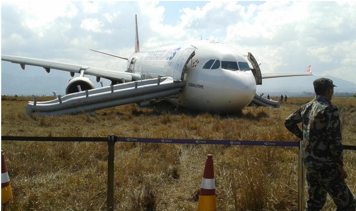
Nose LG collapsed and inserted inside the wheel well
