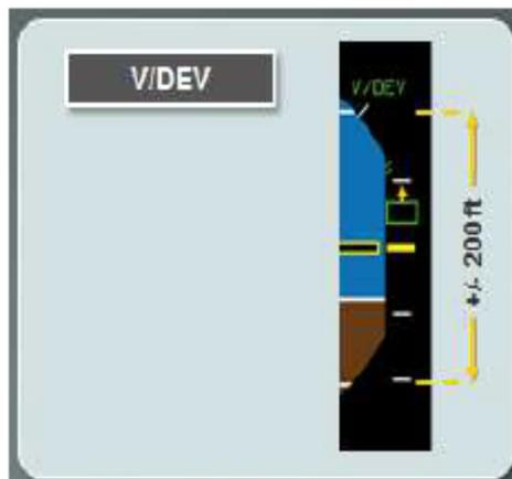
*Note:* According to DFDR, the L/DEV and V/DEV information was displayed on both PFDs during the approach (Ref. DFDR parameters “CLATDEV”, “CVERTDEV” for the captain’s PFD and “FLATDEV” and “FVERTDEV” for the F/O’s PFD).
